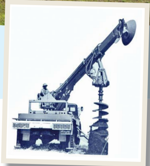
Main: The 10/14 Crane Borer now shares the production line with the Proline LIFT range of vehicle loading cranes. Above: 1965 Proline 3.5/7t Pendulum Borer, Pole Erector. Left: 1962 Proline 6t Articulated Crane Borer.
